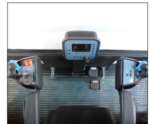
Spill control panel, including arm-rests
